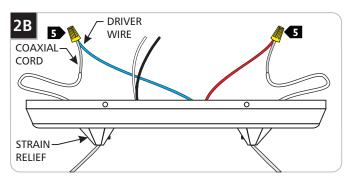
If shortening of the coaxial cords is necessary, take note of the wire connections from the coaxial cables to the driver and remove the wire nuts.
