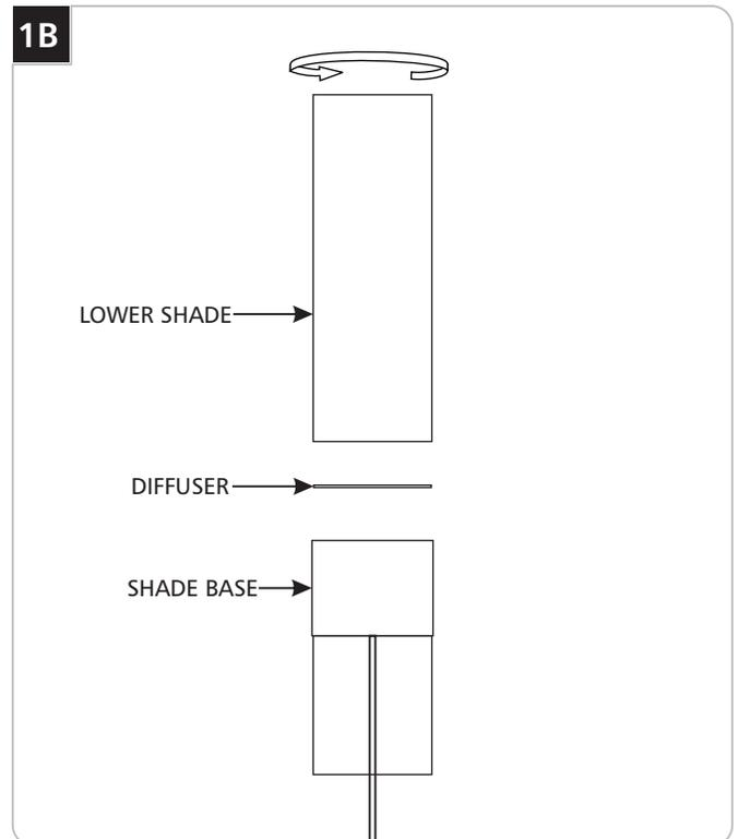
**2** Rotate the fixture upside down, place the diffuser into the shade base, and completely screw the (longer) lower shade into the base.
