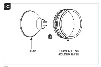
Place the lamp into the louver lens holder base.
