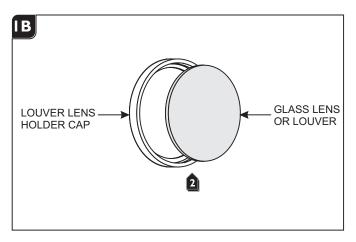
Place the louver or glass lens (optional-not included) into the louver lens holder cap.
