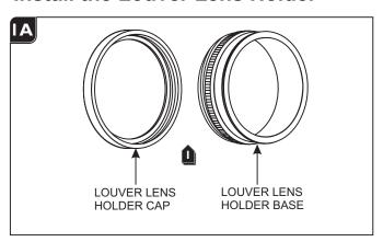
Unscrew the louver lens holder cap from the base.
