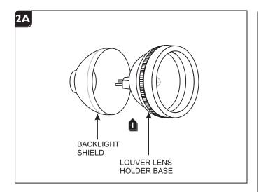
Push the backlight shield onto the louver lens holder base.
